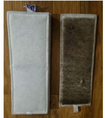
MVHR filters after 3 months
